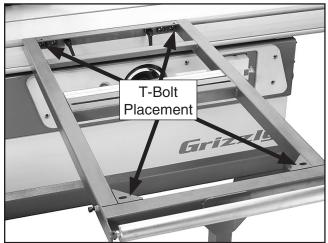
Figure 43. Crosscut fence placement.
